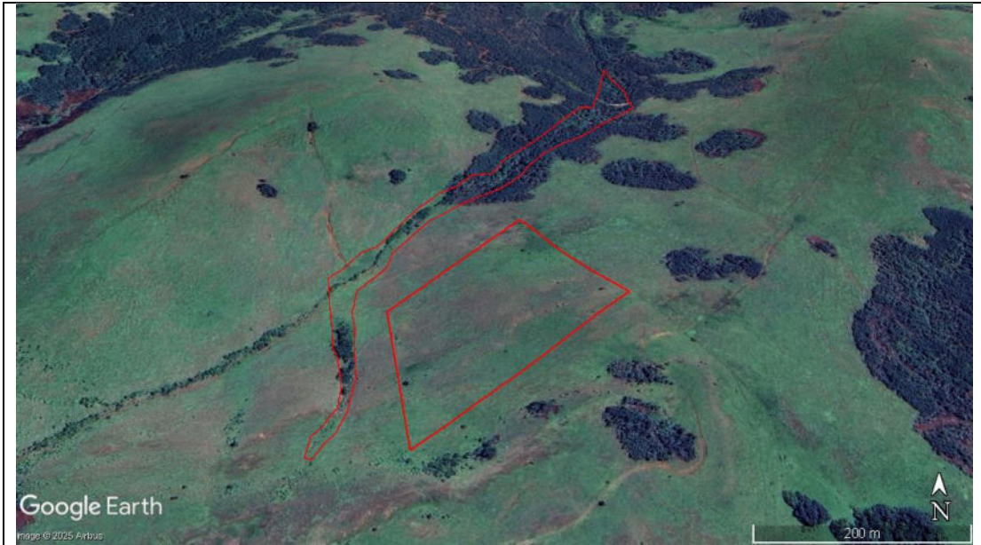
View of Site 1 with the stream visible to the north-west and drainage lines indicated to the south-west. There is a substantial distance between the borrow pit footprint and watercourses. Note also substantial infestation by Acacia mearnsii , especially in the downstream sections.
